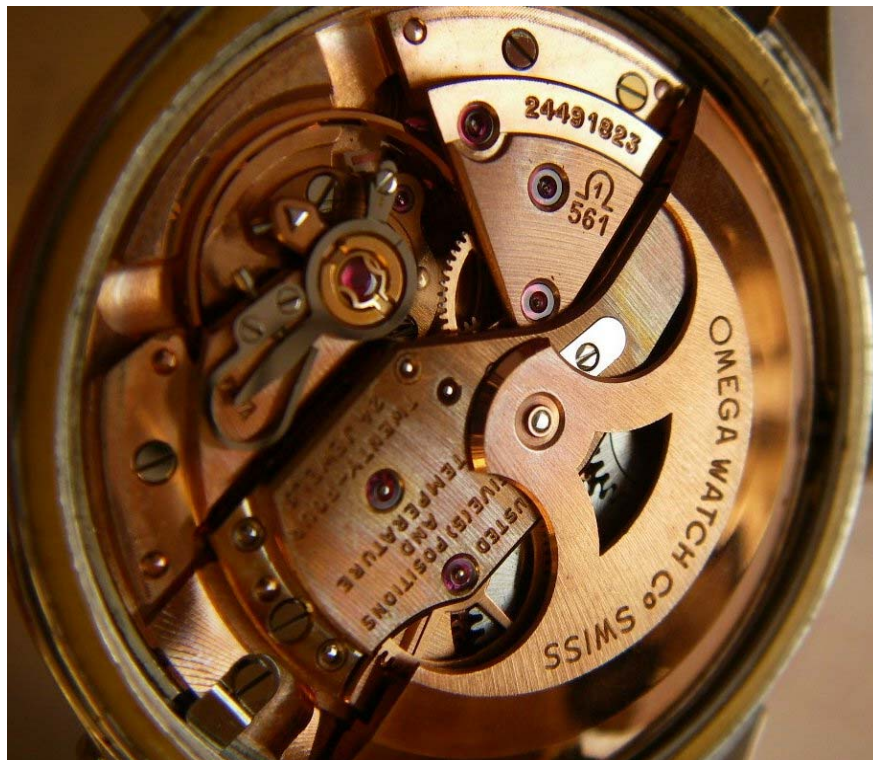
Clean, well-serviced Calibre 561 movement from an Omega Constellation
